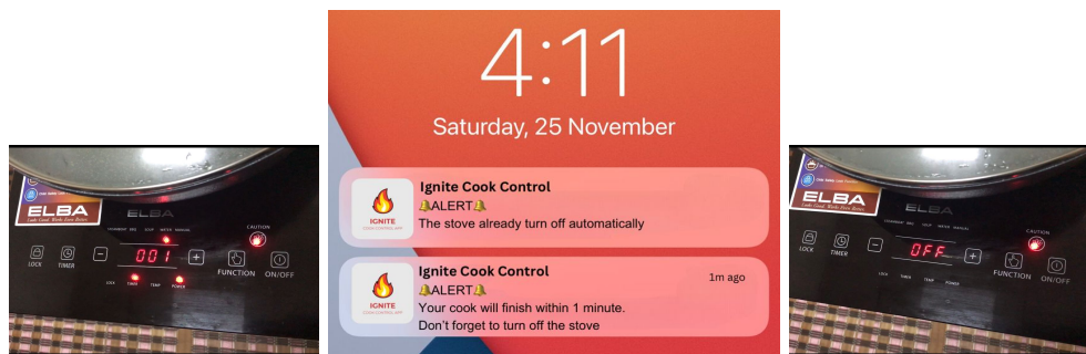
DIAGRAM 5 : Testing Alert (Automatically switch off the stove after the timer finishes)
